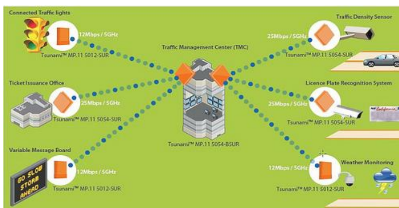
Figure 4. Traffic management in V2I communication
